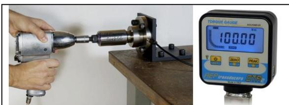
DTR2 + TRF torsionometro STATICO.
