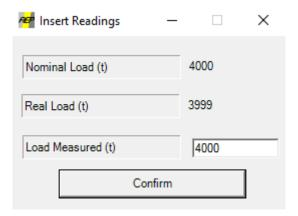
For each measurement point, by pressing the "**Accept the measurement**" button the actual load generated is measured and prompts the operator to enter the load indicated by the machine under test. This value is related to the nominal load required for the measuring point
