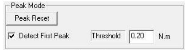
The meaning of the parameter threshold is described in the figure below. It serves to distinguish the actual first peak from any **invalid peak** that may occur during the measurement. In the figure below the point P1 is not valid as the first peak because of the decrease in the next torque was not greater than the established threshold.
