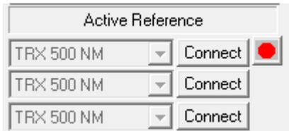
For each torque to be calibrated, a reference instrument can be specified. The reference instrument in use must be connected to the computer through the supplied USB or serial RS232 port. The red dot indicates the active instrument. The correct reference is automatically selected during the test. It is however possible to select the single instrument through the "**Connect**" button.
