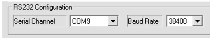
For instruments equipped with a USB port (for example: MP10Plus, MPxPlus, BTR2, DTR2) the Baud Rate can be set at any value.
