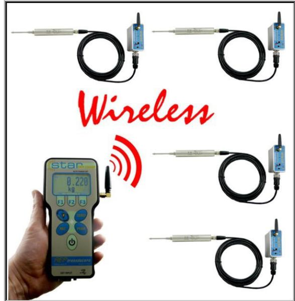
Displacements Monitoring by using LDT transducers.
