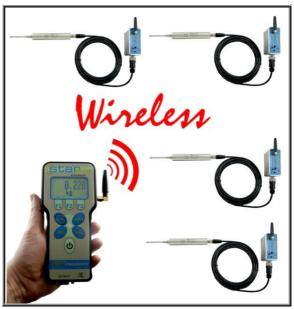
Displacements Monitoring by using LDT transducers.
