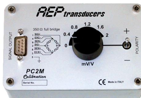
*PC2M signal calibrator has been realised to perform periodical checks and calibrations on indicators with a 2mV/V input and 4 or 6 wires systems.*
