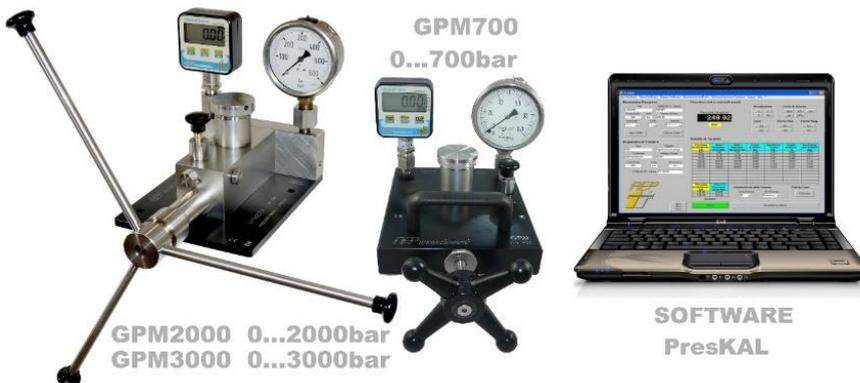
Manual pressure generators used to compare the measurements between the sample manometer and the instrument being calibrated.
